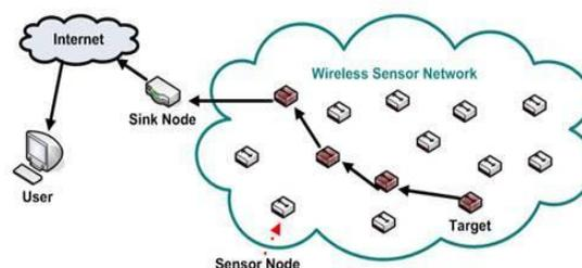
Figure 1. Wireless sensor network configuration
