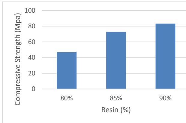
**Figure 5-** Variation of compressive strength with Percentage of Resin
