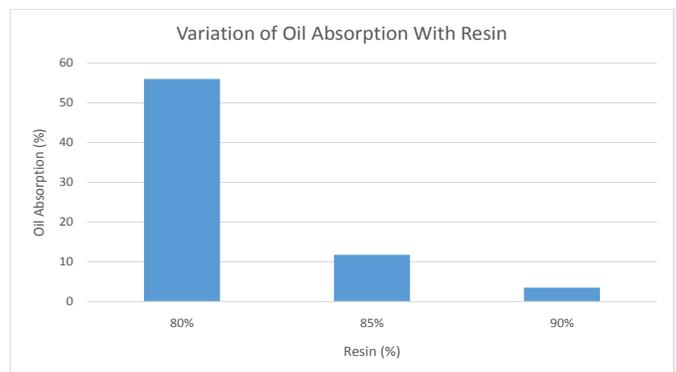
**Figure 8-** Variation Of Oil Absorption With Resin
