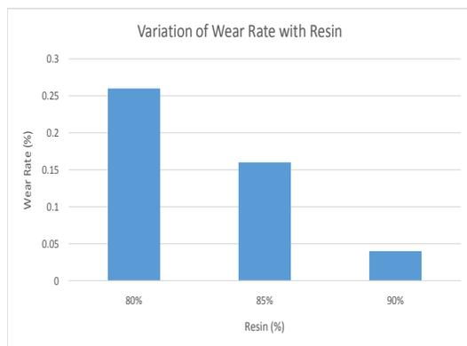
**Figure 6-** Variation of Wear rate with Resin
