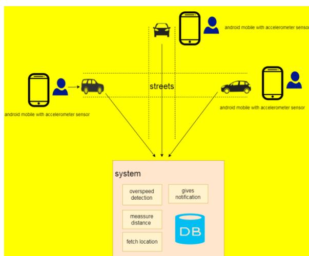
In this user get notification of over-speeding through application, application get information through accelerometer sensor and gives notification “drive slow “if user drive over speed limit or fast. User also gets info. Of nearby vehicles through app. If a vehicle comes toward user from front side/back side or any side then user get notification and its location from user. This location gets through haversine algorithm in system.
